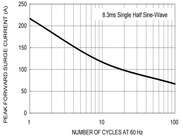
FIG2: Surge Forward Current Capability
