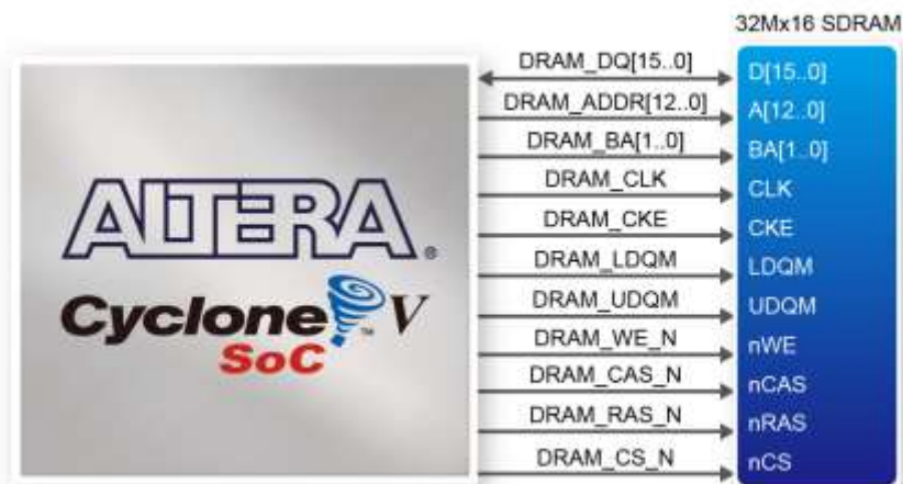
Figure 3-28 Connections between the FPGA and SDRAM
