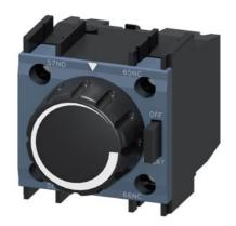
pneumatically time-delayed auxiliary switch, off delayed 1-30 s, 1 NO + 1 NC, for mounting to contactors  $3\mathsf{RT202}$
