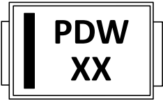
Cathode Band (for uni-directional products only)
