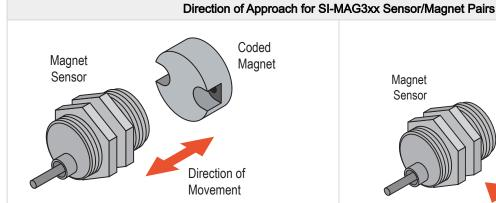
Normal Direction of Approach: movement is perpendicular to the plane of the sensing face.
