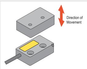
Incorrect Direction of Approach: Label-to-label approach of sensor and magnet is not possible
