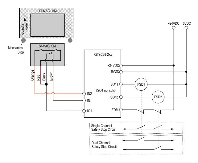
**IMPORTANT:** If the model number of the magnetic switch does not include a letter between the SI-MAG and the number, the orange wire shown is blue and the red wire is gray on older models.
