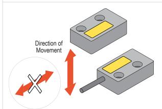
Alternate Direction of Approach: movement is parallel to the plane of the sensing face
