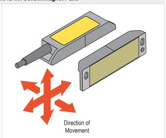
Incorrect Direction of Approach:  $90^{\circ}$  approach of sensor and magnet is only possible with the SI-MAG1MM90 magnet
