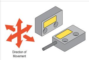
Incorrect Direction of Approach: 90° approach of sensor and magnet is not possible
