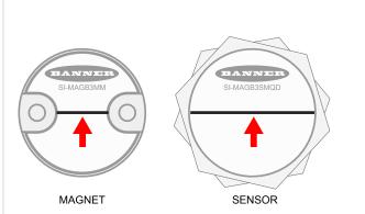
The horizontal line on the magnet face and sensor face shown parallel to each other for optimal performance.
