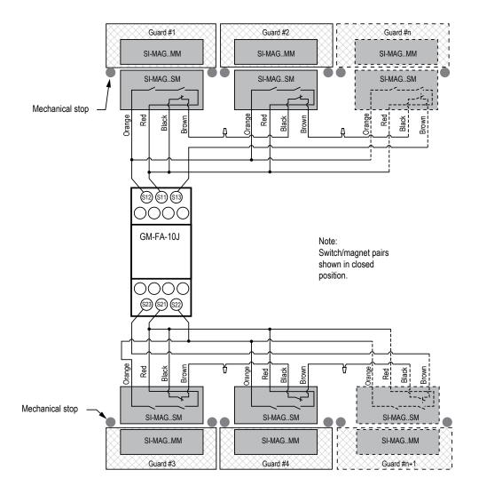
**IMPORTANT:** If the model number of the magnetic switch does not include a letter between the SI-MAG and the number, the orange wire shown is blue and the red wire is gray on older models.
