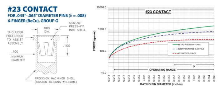
The insertion / extraction force characteristics above were derived using a 30 microinch gold-plated contact and polished steel gauge pins having a bullet-shaped tip.
