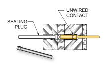
Grommet sealing plugs are used to seal unwired contact cavities. The size #23 sealing plug is specially designed to fit Glenair Series 80 grommets. After installing unwired contacts into unused cavities, insert knob end of sealing plug into grommet until it bottoms against the unwired contact per illustration. Install sealing plugs with standard contact insertion/extraction tools . The size #23 plug is polyphenylsulphone.
