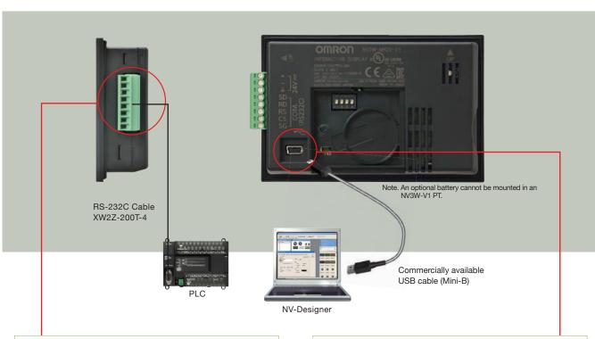
Serial Communications/Power Supply Connector
