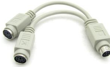
Figure 4-26 Y-Cable use for both Keyboard and Mouse
