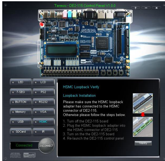
Figure 3-13 HSMC loopback verification test performed under Control Panel
