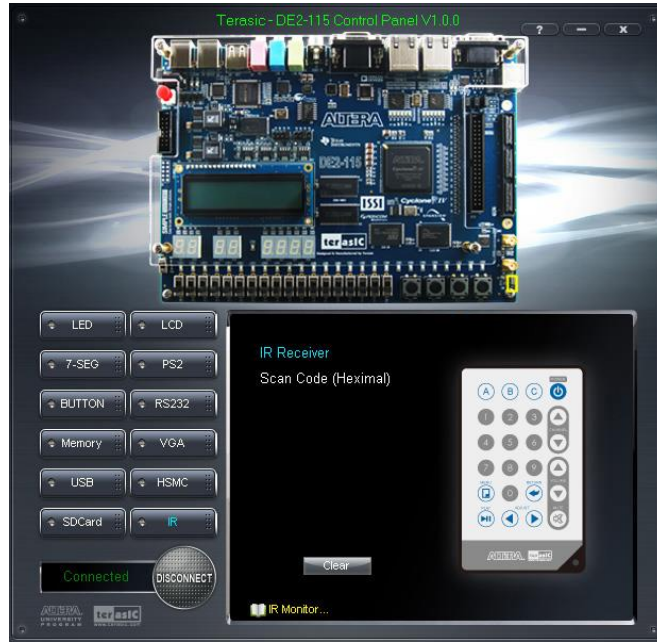
Figure 3-14 Testing the IR receiver using remote controller
