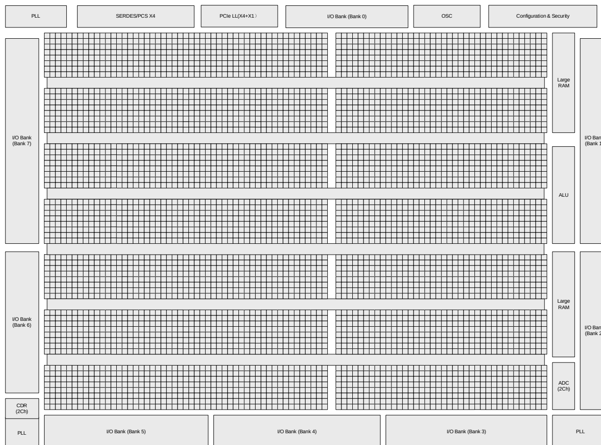
Figure 2.1. Simplified Block Diagram, LFCPNX-50 Device (Top Level)
