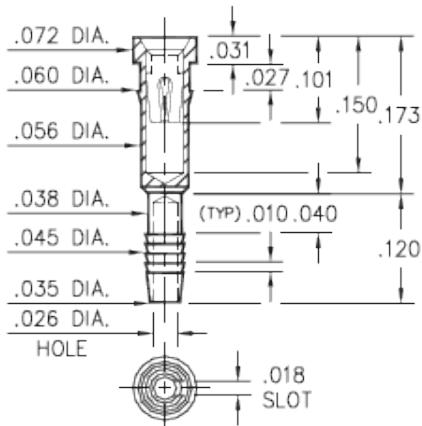
**4612-0-31-XX-30-XX-04-0**Compliant press-fit in  $.040 \pm .003$  plated hole. For  $.060 \rightarrow .100$  thick board**Description:**
