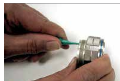
Plastic tool with contact in proper position.
