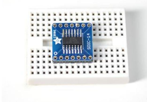
Break two pieces the same length as the pads on either side of the PCB and place them into a breadboard, long pins down. They should be parallel and the same distance as the PCB pads so that you can place the PCB on top with ease
