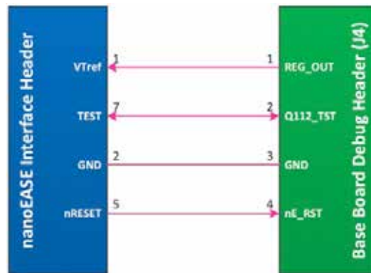
Figure 38: nanoEASE - Base Board Connection Diagram
