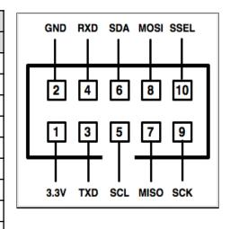
Note that the I2C lines have 10k pullup resistors. SPI1\_NSS also has a 10k pullup.
