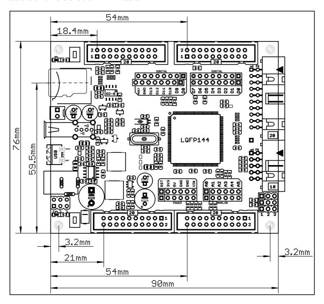
The three highest elements on the board in order from the tallest to the shortest are: capacitor C46 - 17.2 mm (0.677") over the pcb; USB host connectors -14.3 mm (0.563"); capacitors C11 and C3 - 11.5 mm (0.453").
