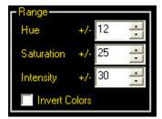
Enter a value or use the arrow keys to specify a tolerance for Hue and/or Saturation. As you adjust the tolerance, it is shown in the Color Map.
