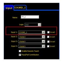
4. Click on the Coordinate Tool (COORD\_1) tab and make sure that the checkmark next to the X-Coordinate value checked. Enter 0 (zero) in the Min column and a lage number (e.g., 1000) in the Max column.
