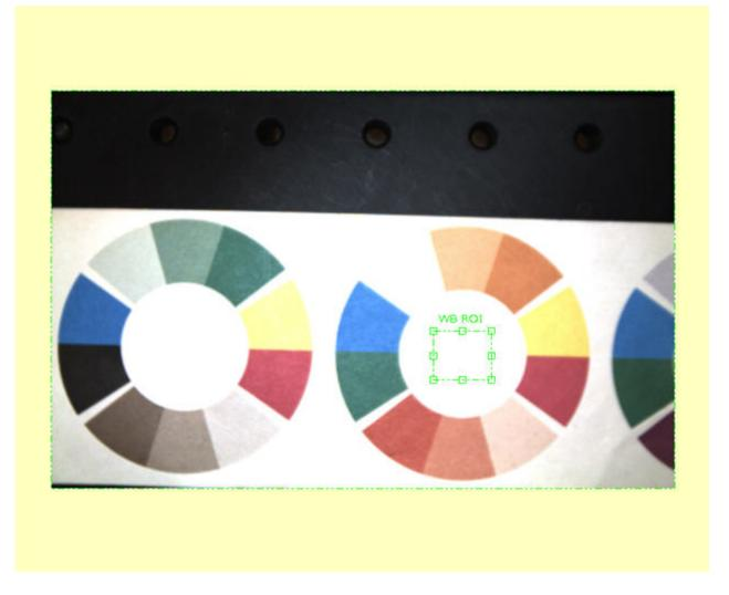
Draw the WB ROI on a region of the image known to be white. This routine will automatically adjust the gain for each of the R, G, and B channels in an effort to make the area in the WB ROI appear white. Strange effects can occur if the area in the WB ROI is not in fact white as shown below when white balancing on blue. This effects will carry over to the gray scale version of the image too.
