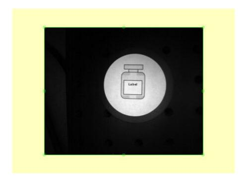
To improve performance, reduce the size of the FOV either vertically, horizontally, or both, as shown below.
