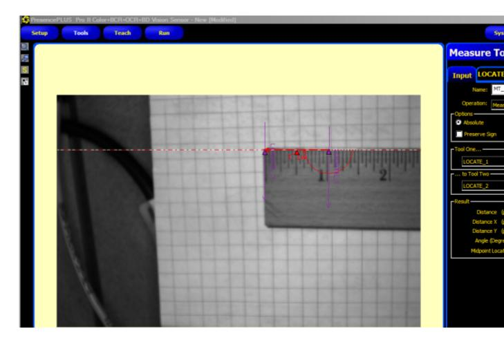
3. In the Units tab, select the desired units and enter the pixel value in the **Measurement in pixels** field.
