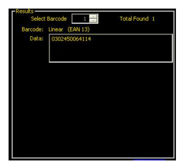
The Results field provides the number of barcodes found, barcode type, data read, and quality parameters.
