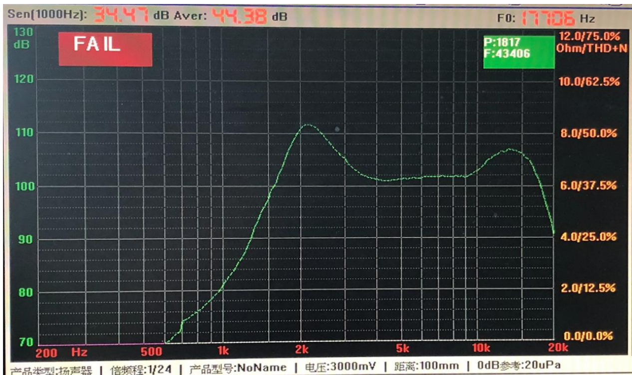
FIG..2(Loud speaker Typical Frequency Response)
