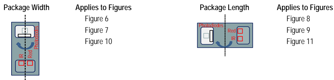
Figure 5. Package Rotation Axes for Field of View
