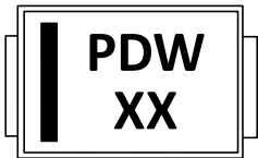
Cathode Band (for uni-directional products only)
