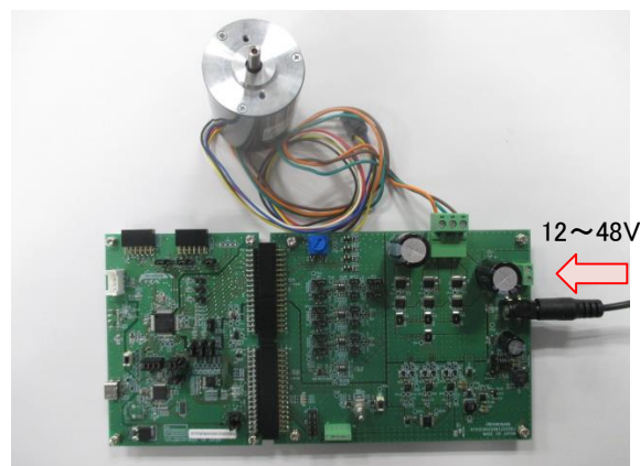
Figure 4-10 Power supply from DC jack
