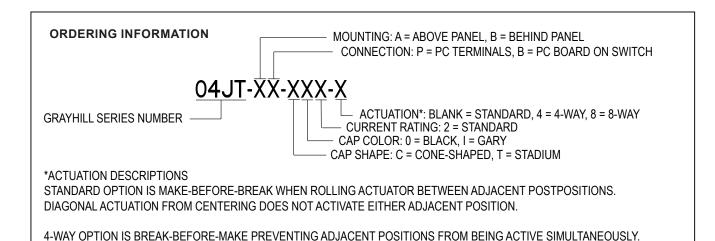
8-WAY OPTION ALLOWS ACTIVATION OF TWO ADJACENT POSITIONS DIRECTLY FROM CENTER WITH DIAGONALLY ACTUATION
