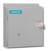
Non-reversing motor starter, Size 2 1/2, Three phase full voltage, Solid-state overload relay, OLRelay amp range 25-100A, 380 440/440 480V 50/60HZ coil, Non-combination type, Enclosure type 12, Dust/drip proof for indoors, Extra-wide enclosure
