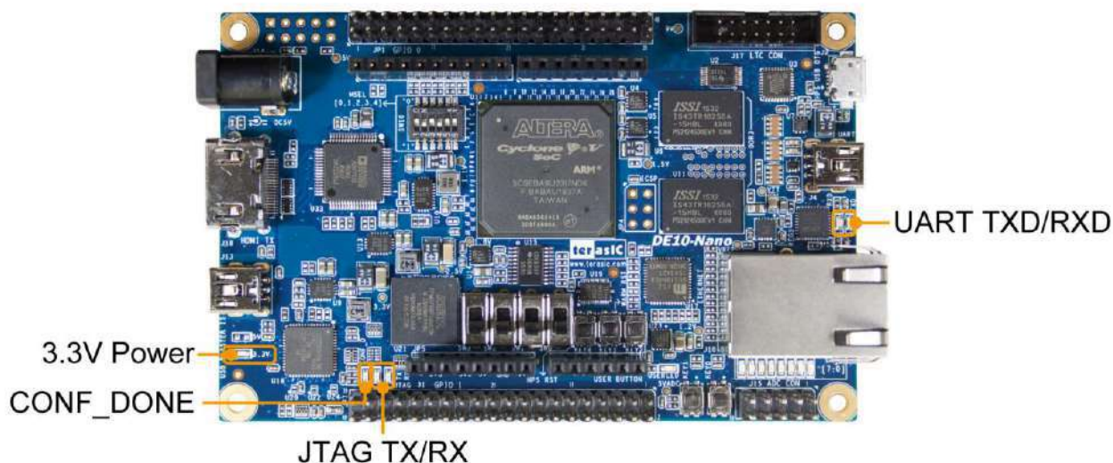
Figure 3-12 LED Indicators on DE10-Nano
