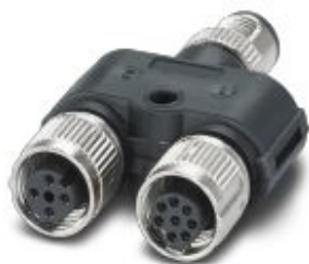
Y distributor for PSR-CT series RFID transponder switches, M12 male/female, 5- and 8-pos., for safe series connection of up to 30 devices
