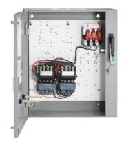
2-speed 3-phase motor starter Size 0 One winding consequent pole Constant or variable torque Solid-state overload relays Low SPD OLR range 0.75-3.4A High SPD OLR range 0.75-3.4A 110-120/220-240VAC 60HZ coil Combination type 30Amp disconnect switch Enclosure NEMA type 1 Indoor general purpose use
