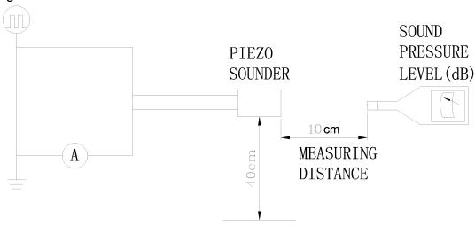
In the measuring test, buzzer is placed as follows:
