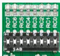
Figure 6-2: Tri-state DIP switch on PORTC
