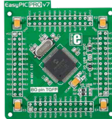
3 Figure 4-7: Standard 80-pin MCU card with PIC18F8722 .
