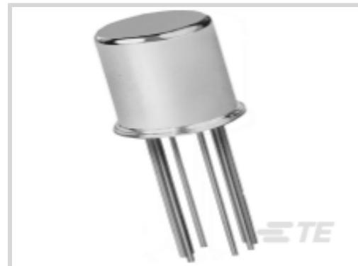
Contact Arrangement: **1 Form C, SPDT, 1 C/O**Input Voltage: **11.6 VDC**Coil Voltage: **18 VDC**Coil Resistance: **2300 Ω**Coil Power Rating DC: **141 mW**
