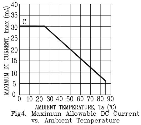
Fig4. Maximum Allowable DC Current vs. Ambient Temperature
