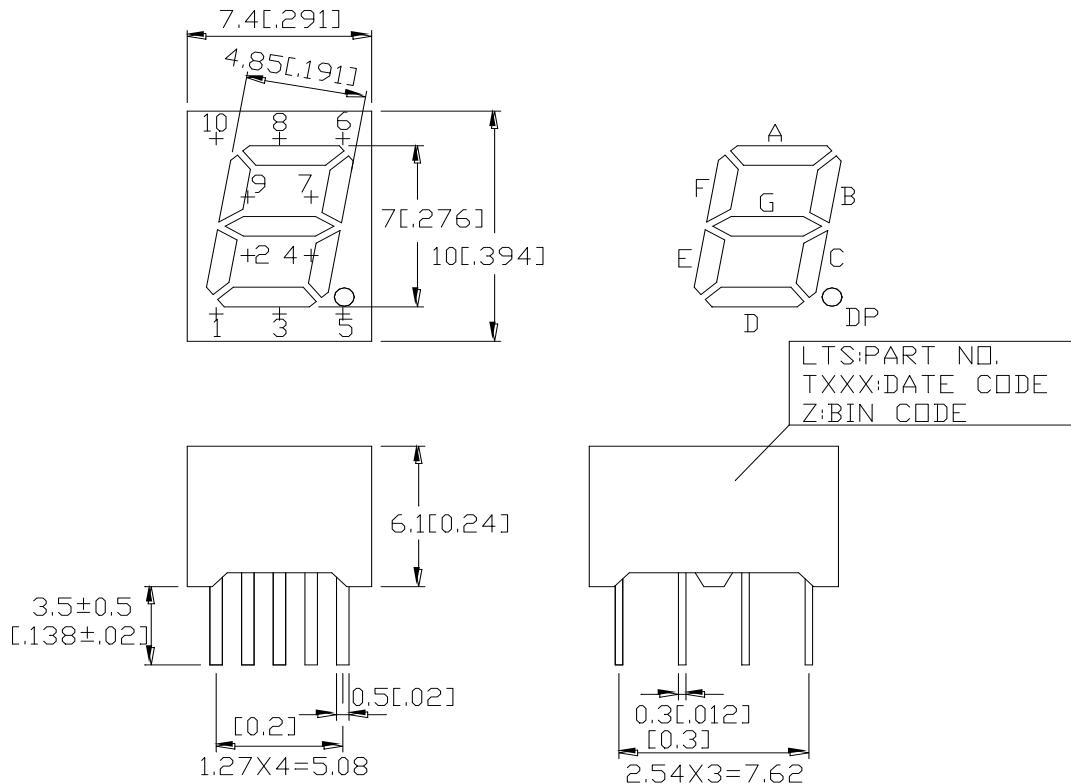
NOTES: All dimensions are in millimeters. Tolerance is  $\pm 0.25$  mm (0.01") unless otherwise noted.
