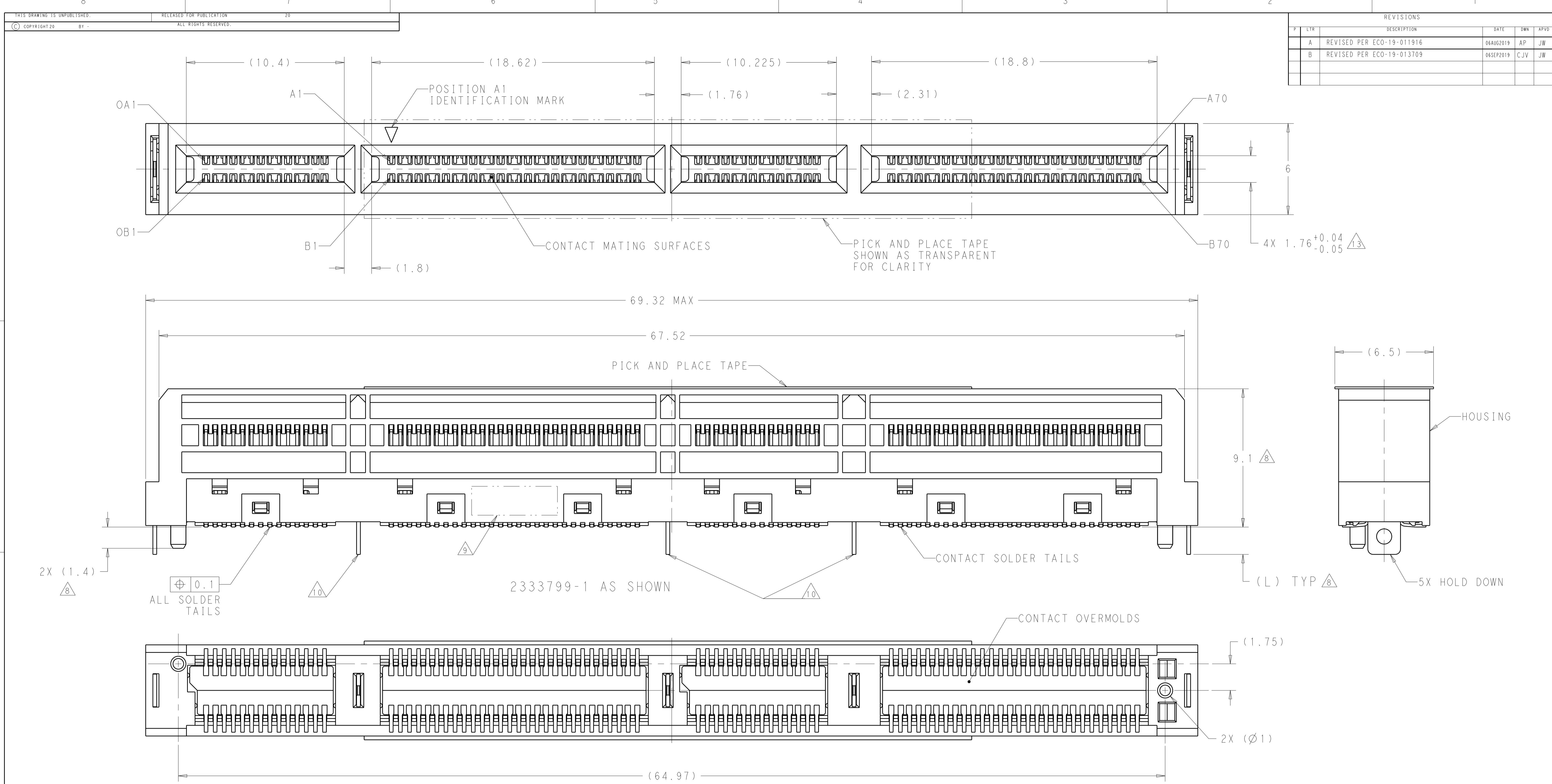
1 HOUSING AND CONTACT OVERMOLDS - LCP, BLACK, UL94V-0 RATED. CONTACTS AND HOLD DOWNS - COPPER ALLOY. PICK AND PLACE TAPE - POLYIMIDE FILM.
