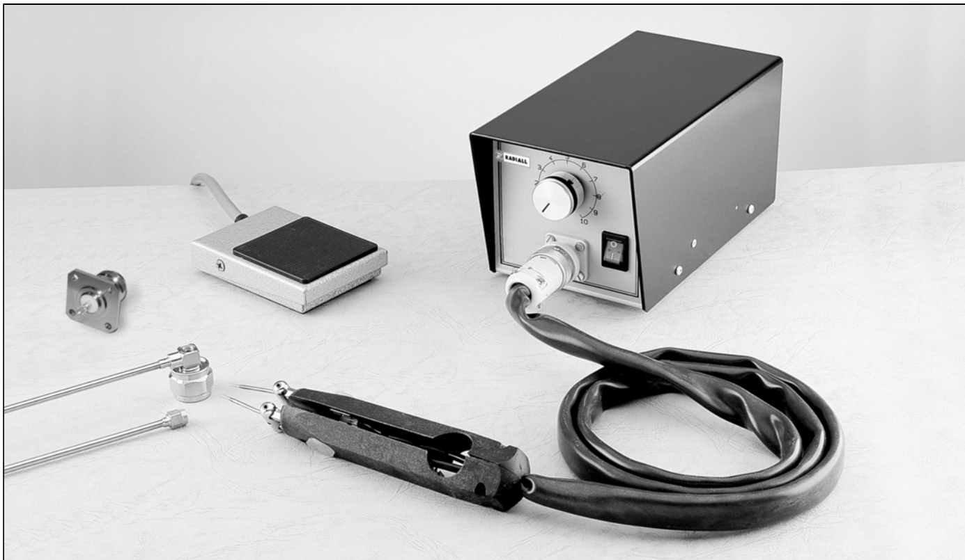
Joule effect soldering device
