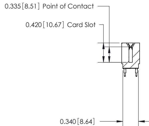
726 Series Ultra-Mate Card Edge Connector - Press Fit
