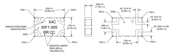
Dimensions are in Inches [Millimeters] X4C30F1-30S Mechanical Outline
