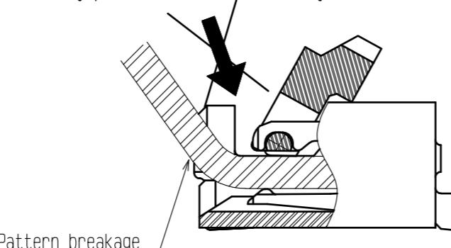
◆Checking the Locking Condition
