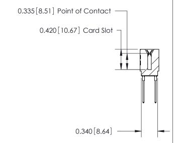
ACAD REFERENCE NO. 726 Series Ultra-Mate Card Edge Connector - Press Fit DRAWN: J.LEE Part Number: 726-020-545-201 CHECKED: **EDAC INC** SCALE: THESE DRAWINGS AND SPECIFICATIONS ARE THE PROPERTY OF EDAC INC.,AND TORONTO, ONTARIO SHALL NOT BE REPRODUCED, OR COPIED DRAWING NUMBER CANADA OR USED AS THE BASIS FOR THE 726-ENG MASTER MANUFACTURE OR SALE OF APPARATUS YOUR CONNECTION TO QUALITY & SERVICE WITHOUT WRITTEN PERMISSION.
