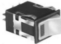
AML34 Series Rocker Switch, SPST, 2 position, Silver Contacts, 0.187 in x 0.02 in (Solder or Quick-Connect), 1 Lamp Circuit, Rectangle, Snap-in Panel
