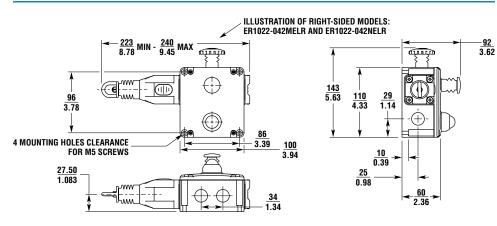
Note: The designation of the ER1022 switch as left-sided or right-sided is based upon the mounted position of the switch, in the installation.
