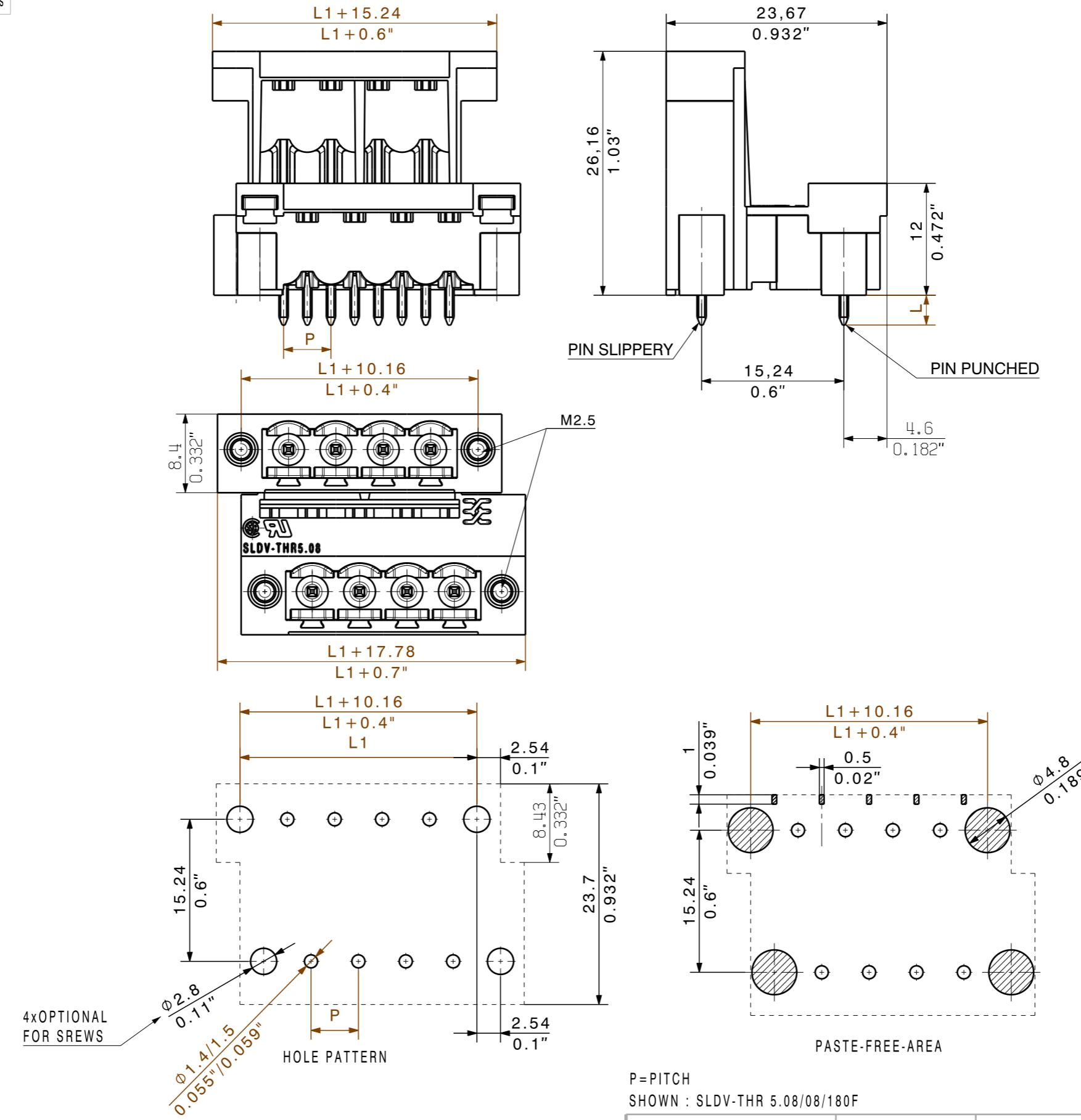
For the mounting of PCBs, it should be noted that the rated data given in the catalogue relates only to the connection elements. The necessary creepage and clearance paths must be observed in connection with the respective applicant in accordance to VDE 0110. The current-carrying capacity and pitch tolerance is to be determined according to DIN IEC 326 part 3 very fine.
