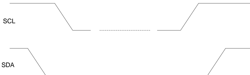
Figure 21: I 2 C START and STOP Condition Timing
