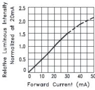
Fig.4 RELATIVE LUMINOUS INTENSITY VS. FORWARD CURRENT
