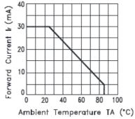
Fig.3 FORWARD CURRENT DERATING CURVE
