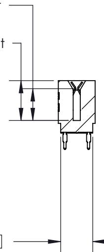
726 Series Ultra-Mate Card Edge Connector - Press Fit
