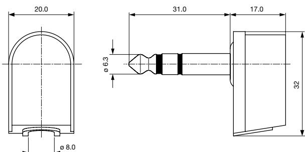
Cable diameter max. 8.0 mm
