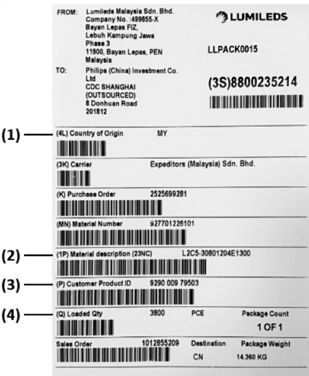
Figure 14. Example of outer box label for LUXEON CoB Core Range with CrispColor Technology.
