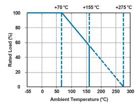
For resistors operated in ambient temperatures above  $70^{\circ}$ C, power rating must be derated in accordance with this curve.
