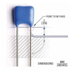
Very often before soldering through-hole components, their leads get bent. It is important not to damage the components during lead bending. Damage most commonly incurred during bending is cracks in epoxy parts, which can lead to increased humidity sensitivity of a component and, consequentially, a shorter lifetime.
