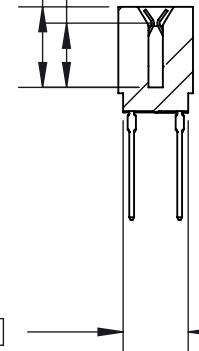
726 Series Ultra-Mate Card Edge Connector - Press Fit
