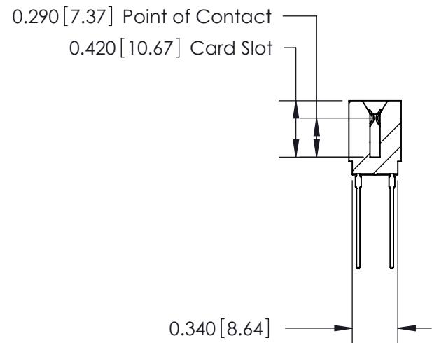
726 Series Ultra-Mate Card Edge Connector - Press Fit
