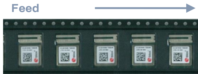
Figure 13: Orientation of NINA-B112 modules on tape
