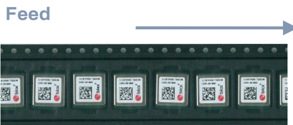
Figure 12: Orientation of NINA-B111 modules on tape
