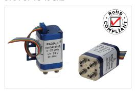
Radiall's TITANIUM series switches are optimized to perform at a high level over an extended life cycle. With outstanding RF performance, and a guaranteed insertion loss repeatability of 0.03 dB over a life span of 2.5 million switching cycles. Radiall's TITANIUM switches are perfect for automated test and measurement equipment, as well as signal monitoring devices.
